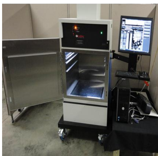
Fig 1. The “protected” training-research X-ray unit for distance education for medical physics students.
