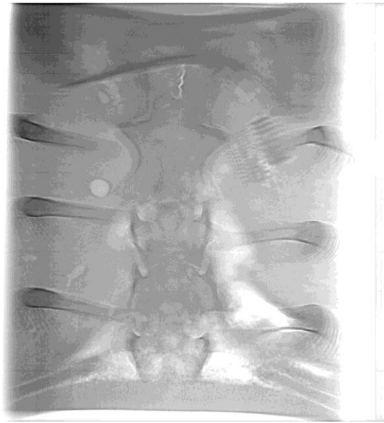
Fig. 4. Section of the paraffin phantom, obtained with prototype tomosynthesis unit. Section is reconstructed from 29 projections every 1^\circ in range -14^\circ \dots +14^\circ . Dimensions are 3024x3024 pixels, intensity varies in range 8000...45000.
