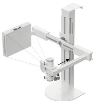
Figure 1. UNIMAT TOMO X-ray stand with IONA2-RF-4360 digital detector and tomosynthesis mechanical adapter. Source-to-image plane distance is 1400 mm, scanning angle is 30°.
