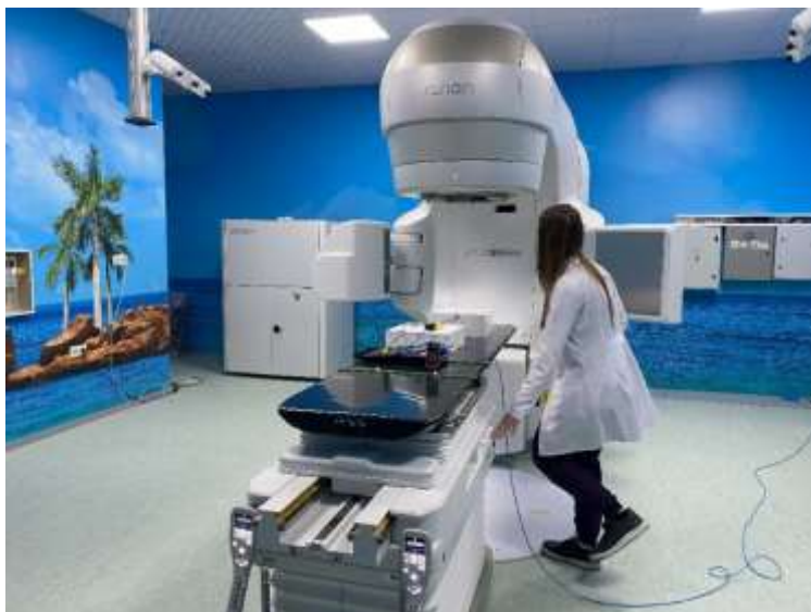
Fig. 3. Demonstration of output constancy check with solid water phantom as part of linac daily
